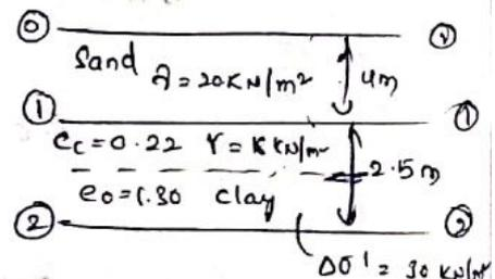
$$\Delta H = \frac{H \times \gamma_w}{1 + e_0} \times \log_{10} \left( \frac{\sigma_1}{\sigma_0} \right) \quad (\sigma_1 = \sigma_0 + \Delta \sigma_1)$$
