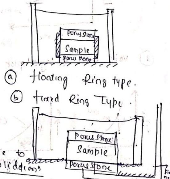
The decrease in the vol of soil due to expulsion of water is called "consolidation"
