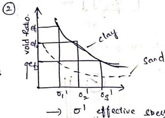
③ void ratio  $v$  vs  $\log \sigma'$  plot
